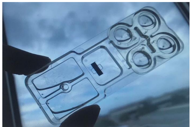
Figure 4. Picture of the current cartridge design, with the waste reservoirs containing corresponding waste after running an assay.
